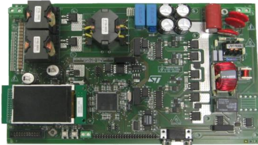
Figure 8: STEVAL-ISV003V1, 250 W microinverter for plug-in PV panels
