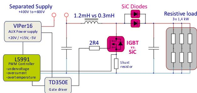
Fig. 4 4kW DC/DC boost converter developed in our laboratory
