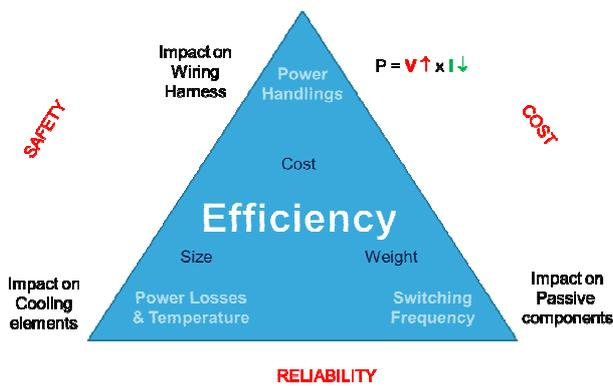
Fig. 1 Power semiconductor challenges for EV and HEV
