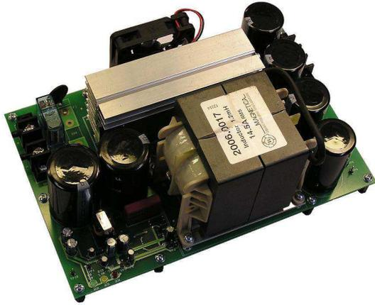
Fig. 3 4kW DC/DC boost converter developed in our laboratory
